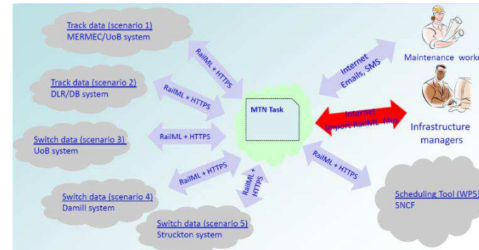
Man-machine interface to help maintainers and link to the planning & scheduling tool (Deliverable 3.2 p 36)
