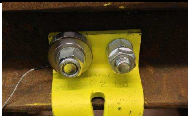
Figure 16 - Test example of a smart washer at the University of Birmingham
